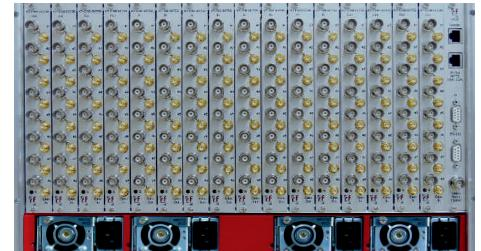
Additional flexibility is being provided via available options like switchable LNB-supply for each input while this option also allows insertion of an external 10Mhz signal.
