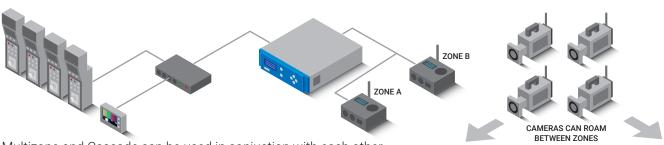
Multizone and Cascade can be used in conjuction with each other, making a complex network with very large coverage potential
