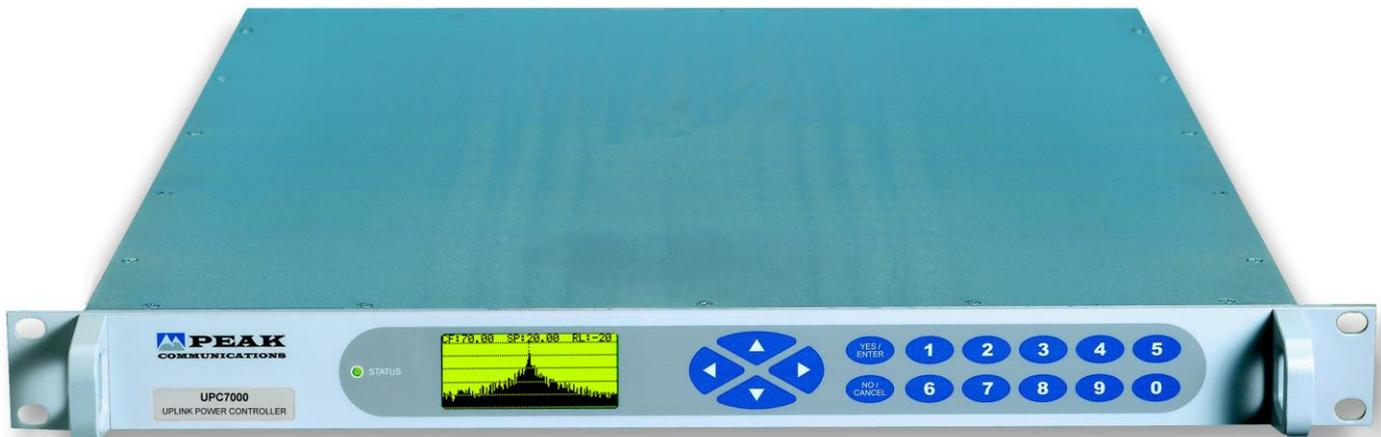
The **UPC7000 series** are next generation automatic UpLink power control units (AUPC's) that measure the 'link loss' from a satellite beacon signal and subsequently automatically control the UpLink power via a number of adjustable IF or L-Band channels. As standard the system is 'lossy' (unity gain at minimum attenuation) and based on electronically variable attenuation, however system gain can be added to overcome external system & cable losses, if required.
